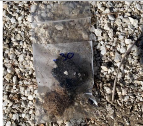
Photo of HA number 10, Non-ACM BUR Roof Core with Gravel, Throughout Roof Except Foam Core
