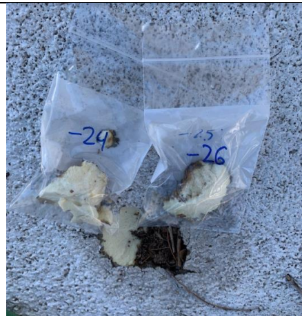
Photo of HA number 8, Non-ACM Foam Roof Core with White Texture Coat, Throughout Floors Under Tiles of Crafts Room, Office and Storage
