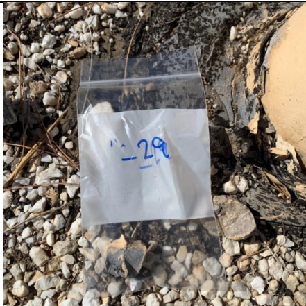
Photo of HA number 9, ACM Black Roof Penetration Mastic, Throughout Roof Penetrations
